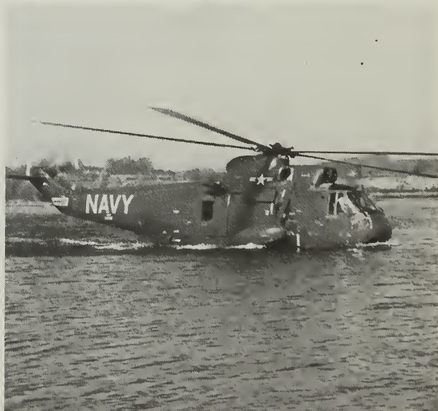
WATER BIRD —New gas-turbine-powered copter with choice of boat hull or wheels can land almost anywhere.
